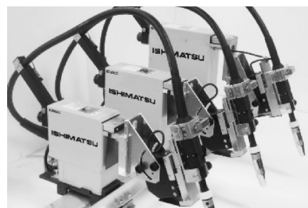
Fig. 5 Compact portable welding robot ISHIMATSU™
