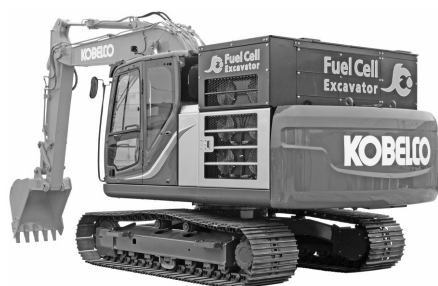
Fig.13 Fuel Cell Excavator
