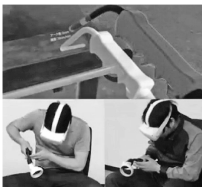
Fig.21 Virtual welding training system “NAP welding training”
