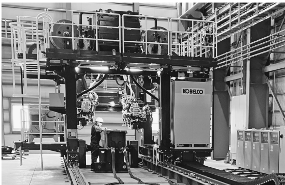
Fig. 9 Example of Kobe Steel's multi-electrode submerged arc welding system for corner joints of built-up box section column (Customer: OATEC corporation)
