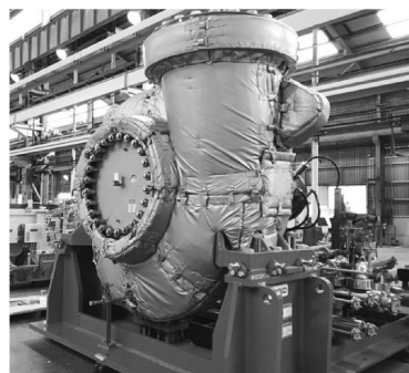
Fig. 5 Centrifugal compressor for EO/EG application
