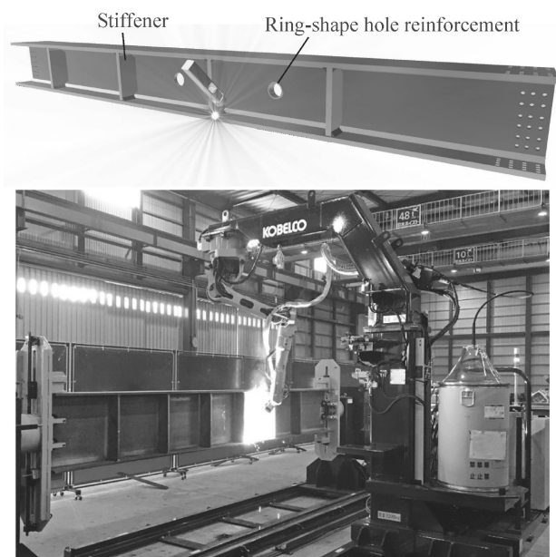
Fig.17 Welding of beam parts and “ARCMAN™” steel frame welding robot system for H-beam assembly
