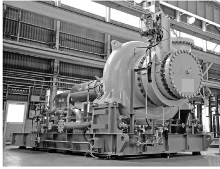
Fig. 6 Centrifugal compressor for PDH application
