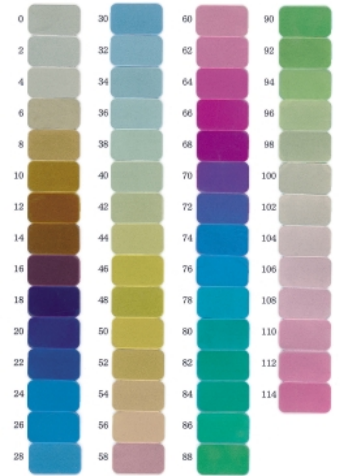
Fig.27: Appearance of anodized titanium (The numerals show the applied anodizing voltages)
