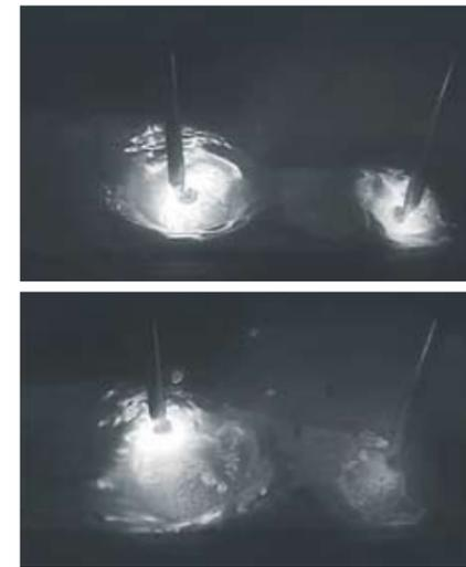
With SENSARC™ AB500, the high quality load-characteristic control reduces spatter generation by as much as 70% as well as spatter particle size, when compared with a conventional power source, as shown in Figure 11.
