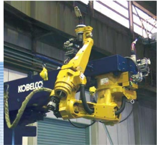
A dedicated welding power source for robots: SENSARC™ AB500
