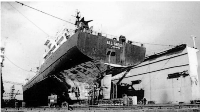
**Fig. 1 — Unithai 1: a floating dock with a docking capacity of 140,000 dwt vessels contains a ship under repair.**
