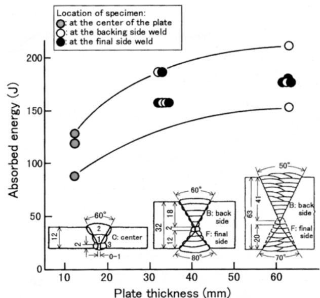
Fig. 2 — Charpy impact test results of LB-52NS (4 mm $\varnothing$ ) weld metals in vertical-up AC welding (interpass temperature: 100-150°C, test temp: -45°C).
