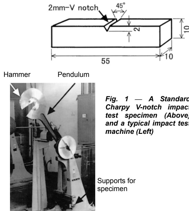
**Fig. 1 — A Standard Charpy V-notch impact test specimen (Above) and a typical impact test machine (Left)**
