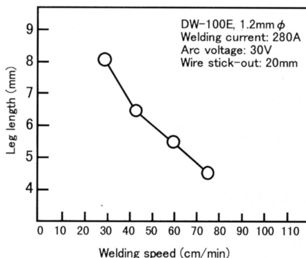
**Fig. 4 — Leg length vs. welding speed in use of DW-100E in single pass horizontal fillet welding**
