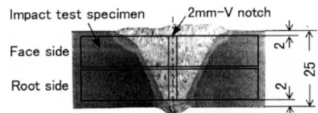
**Fig. 1 — Location of impact test specimens removed from DW-100E welds (One-side welding with FBB-3)**
