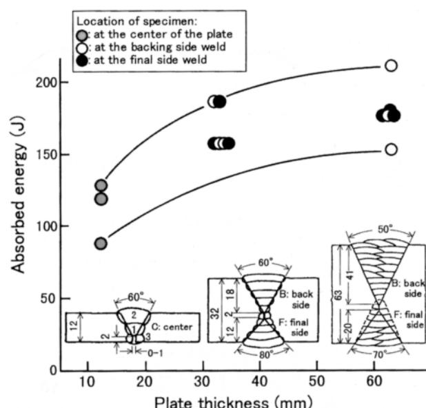
**Fig. 2 — Charpy impact test results of LB-52NS (4 mmØ) weld metals in vertical-up AC welding (interpass temperature: 100-150°C, test temp: -45°C).**
