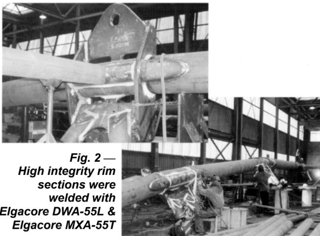
**Fig. 2 — High integrity rim sections were welded with Elgacore DWA-55L & Elgacore MXA-55T**
