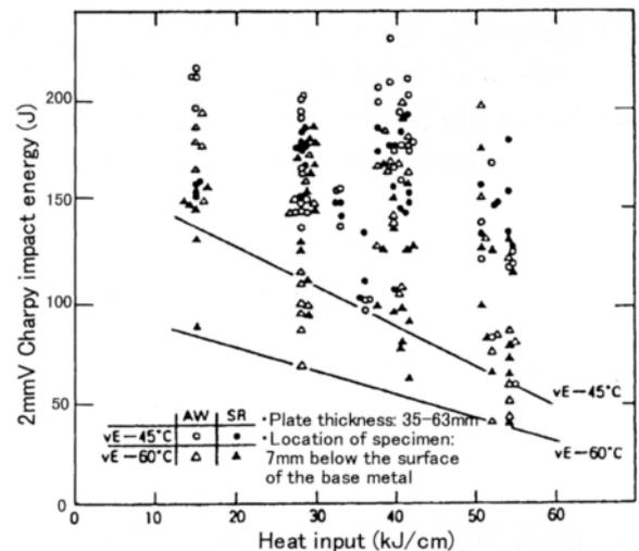
Fig. 1 — Charpy impact absorbed energy of LB-52NS weld metals as a function of heat input in welding thick-section butt joints
