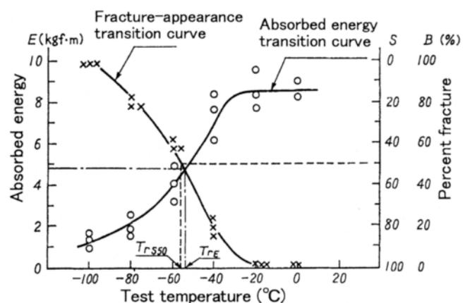
Fig. 2 — Typical transition temperature curves of a carbon or low alloy weld metal (S: shear, B: brittle)
