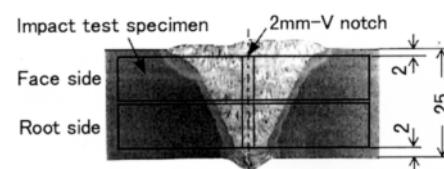
**Fig. 1 — Location of impact test specimens removed from DW-100E welds (One-side welding with FBB-3)**
