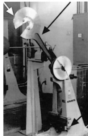
Fig. 1 — A Standard Charpy V-notch impact test specimen (Above) and a typical impact test machine (Left)
