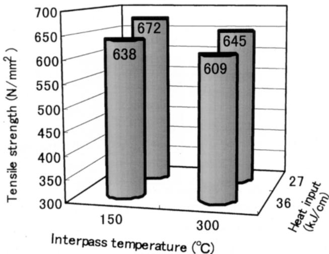
Fig. 4 — The effects of heat input and interpass temperature on tensile strength of MG-60 all-deposited metal
