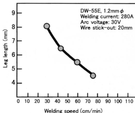
Fig. 4 — Fillet leg length vs. travel speed in use of DW-55E in single pass horizontal fillet welding
