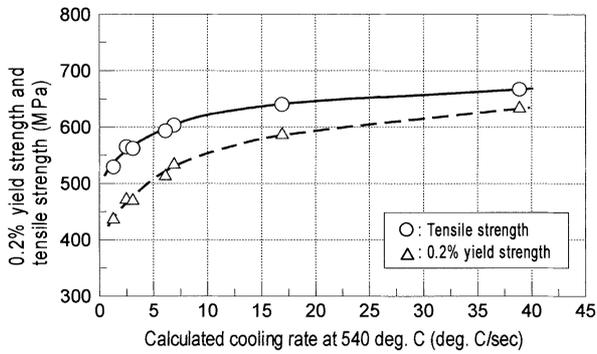
**Fig. 7** 0.2% yield strength and tensile strength of DW-55E weld metal as a function of cooling speed
