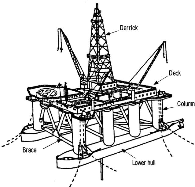
Fig. 5 Columns, braces and lower hulls are the main structural components of a semi-sub rig
