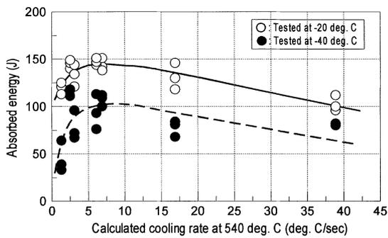
**Fig. 8** Charpy impact absorbed energy of DW-55E weld metal as a function of cooling speed
