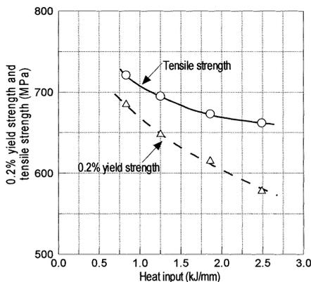
**Fig. 1** Tensile strength and 0.2% yield strength of DWA-65L all-weld metal vs. heat input 1.2 mm wire 280Amp./28-30Volt Flat welding position 80%Ar-20%CO<sub>2</sub> 8-25 passes/5-8 layers Preheat & interpass temp.: 150
