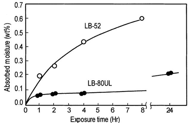
Fig. 6 Moisture absorption curves of LB-52 (E7016) and LB-80UL (E11016-G) tested in the controlled atmosphere (30 × 80%RH)
