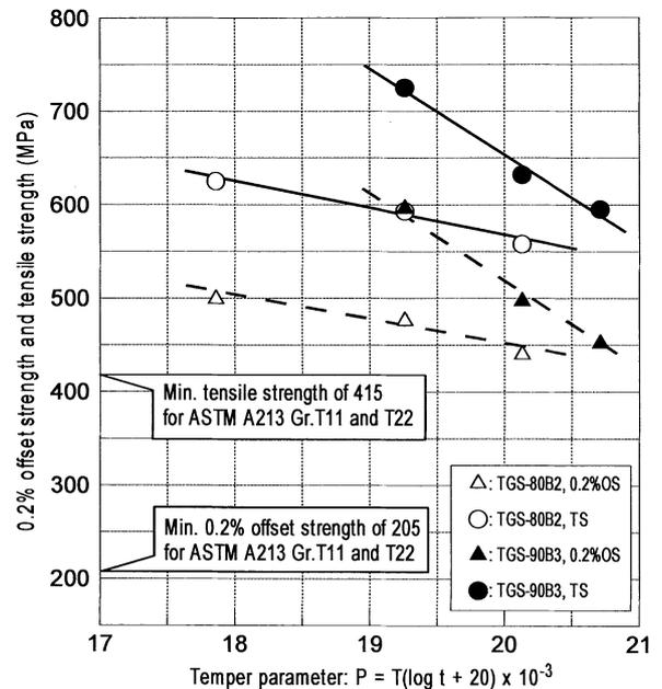
**Fig. 1** Mechanical properties of the all-weld metals of TGS-80B2 and TGS-90B3 as a function of PWHT
