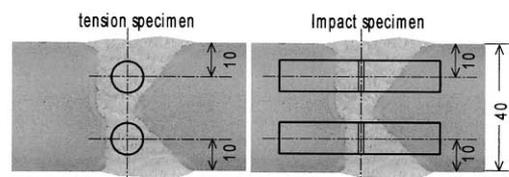
**Fig. 4** Locations of test specimens
