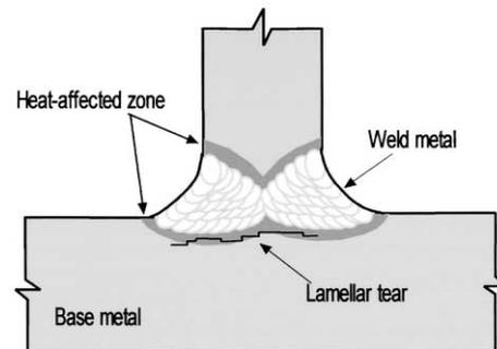
Fig. 2 Schematic lamellar tearing occurring at the area close to the fusion line in the base metal of a node joint
