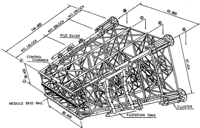
**Fig. 1** Jacket of braced tubular steel structure in the as-fabricated condition
