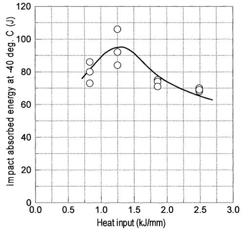
**Fig. 2** Impact absorbed energy of DWA-65L all-weld metal vs. heat input 1.2 mm wire 280Amp./28-30Volt 80%Ar-20%CO<sub>2</sub> Flat welding position 8-25 passes/5-8 layers
