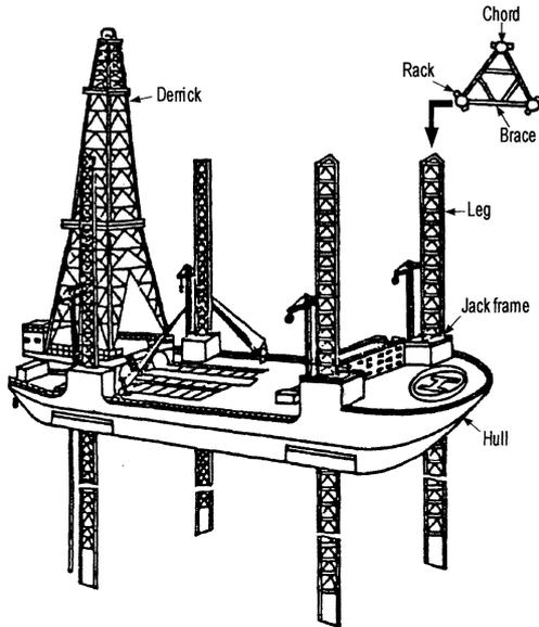
Fig. 3 Legs of a jack-up rig consist of rack, chord, and brace
