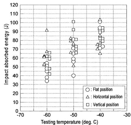
**Fig. 3** Impact test results of DWA-65L joint weld metals
