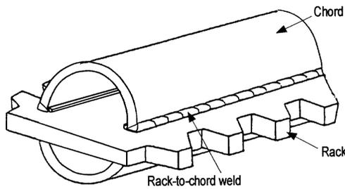
Fig. 4 Rack-to-rack joints are butt welded by SAW, and rack-to-chord joints are butt welded by SAW and GMAW
