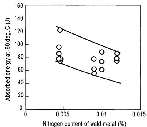
**Fig. 10** Effect of nitrogen in DW-55L weld metal on Charpy impact absorbed energy
