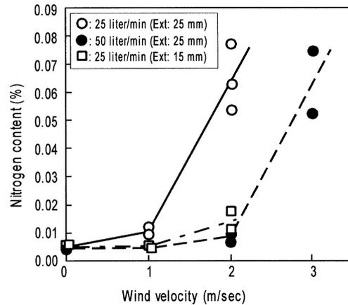
**Fig. 9** Effects of wind velocity on nitrogen content of DW-55L weld metal
