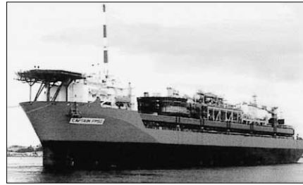
Photo 1. A Floating production, storage and offloading vessel (FPSO) (Source: Fene Shipyard, Italy)
