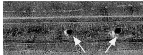
Porosity (pits) appeared in the surface of a weld bead
