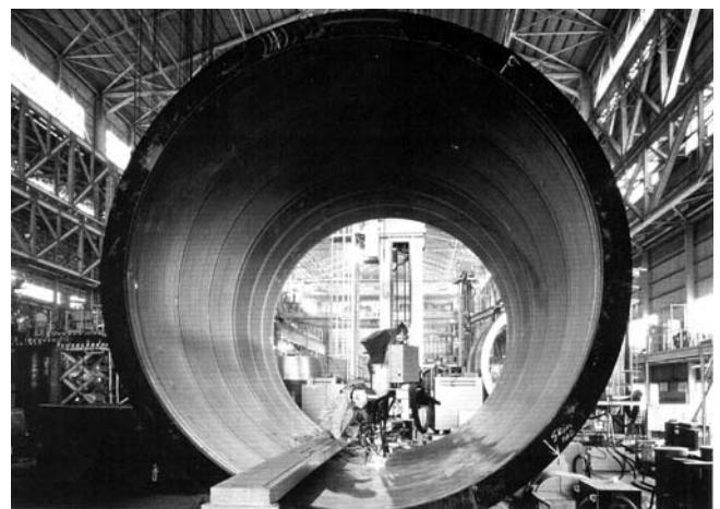
Figure 3: Band-Overlaying of the inside of a shell
