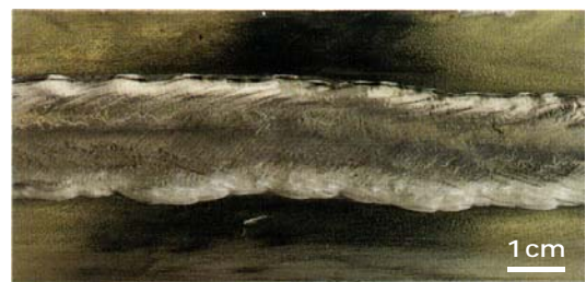
Figure 2: Metallic, lustrous appearance of a weld bead brushed with a stainless steel wire brush
