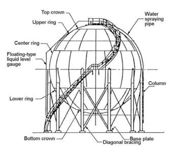
Figure 2: Spherical LPG storage tank.
