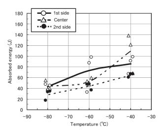
Figure 1: Charpy V-notch impact test results of a weld joint made with LB-7018-1 (3.2 and 4.0 mmØ) and SM490A base metal (50-mm thick double-V groove) in the vertical position. (Heat input: 2.5-2.9 kJ/mm).
