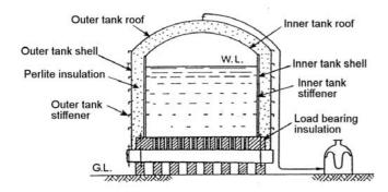
Figure 3: Cross sections over flat-bottom double-wall cylindrical tank.
