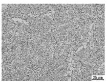
Figure 2: Fine grain microstructure of LB-7018-1 weld metal (as-cast zone) obtained from the 1st side of the 50mm thick double-V groove weld joint.
