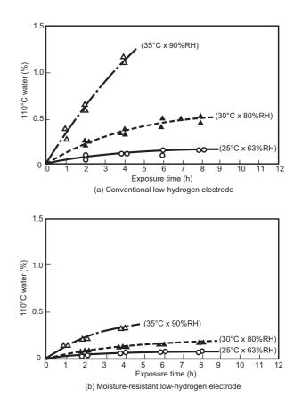
Figure 6: Moisture absorption curves of a moisture-resistant low-hydrogen electrode and a conventional low-hydrogen electrode tested under conditions of controlled temperature and relative humidity.
