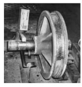
Figure 8: A wheel made of low alloy steel as a typical application for **DWH-250** fluxcored wire of pearlite type.
