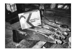
Figure 9: A crusher arm of mild steel, a typical application for **DWH-800** flux-cored wire of the boron martensite type.
