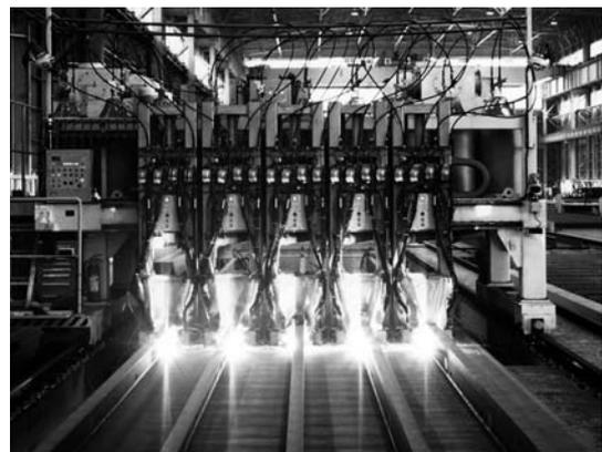
Figure 9: Twin tandem welding of five longitudinals onto one panel by using **MX-200H** flux-cored wires.
