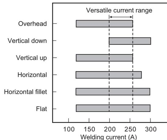
Figure 2: Proper welding current ranges for individual welding positions and versatile current range for positional welding (DW-100, 1.2Ø, CO<sub>2</sub> shielding).
