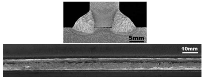
Figure 8: Typical bead appearance and macrostructure of **MX-200H** (1.6 mmØ) fillet weld made by the TOP process on a primer coated steel plate (CO<sub>2</sub> shielding; inorganic zinc primer of approx. 20 µm thick.; travel speed of 150 cm/min.)
