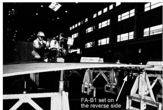
Figure 6: FAB process being used on a curved work with **FA-B1** attached on the reverse side of the work.
