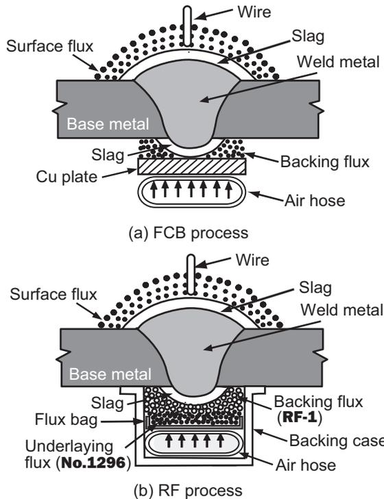
Figure 2: Principles of FCB and RF processes for plate-to-plate one-sided SAW.
