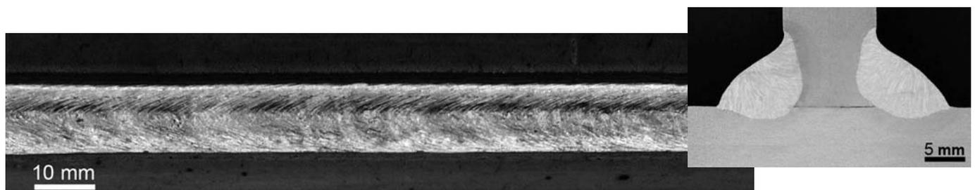
Figure 2: Bead appearance and macrostructure of MX-200E fillet weld made on inorganic-zinc-primer-coated steel fillet joint.
