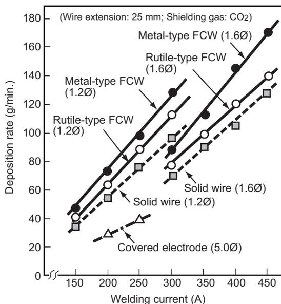
Figure 1: Deposition rates of covered electrodes, solid wires, rutile-type FCWs, and metal-type FCWs as a function of welding currents.
