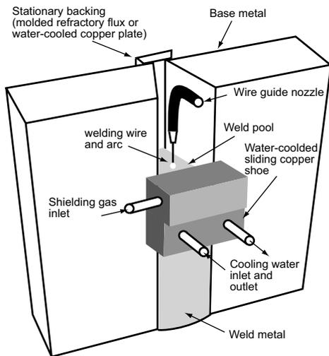
Figure 10: Principles of the SEGARC process for EGW of vertical joints of 9-25 mm in thickness and 2-6 m in length.
