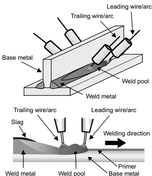
Figure 7: Principles of the Twin-Tandem One-Pool process
