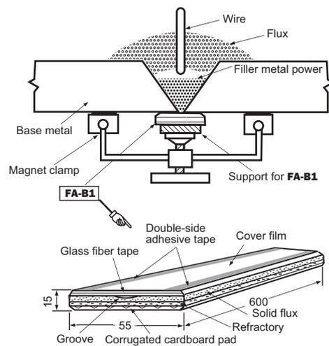
Figure 5: Principles of FAB process with **FA-B1** backing material for one-sided SAW of curved shells and unit blocks.
