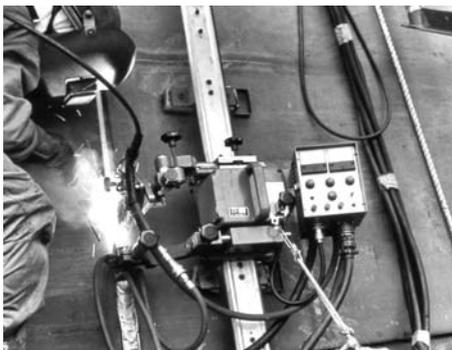
Figure 11: The SEGARC process being used for EGW of a vertical hull joint.
