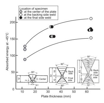
Figure 3: Charpy impact test results of LB-52NS (4.0 mmØ) weld metals in vertical-up AC welding (interpass temperature: 100-150°C).
