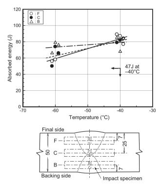
Figure 1: Charpy impact properties of LB-80L (4.0mmØ) weld metal (Base metal: 50-mm-thick 780-MPa high tensile steel of K-TEN780 with double-V groove; Welding position: Vertical-up; Welding parameter: 120Amp./22V; Heat input: 2.0kJ/mm; Preheating and interpass temperature: 150°C).
