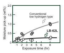
Figure 4: Test results of LB-62L and conventional low-hydrogen electrode on moisture pick-up under the controlled atmosphere:  $30^{\circ}C \times 80\%$ RH.
