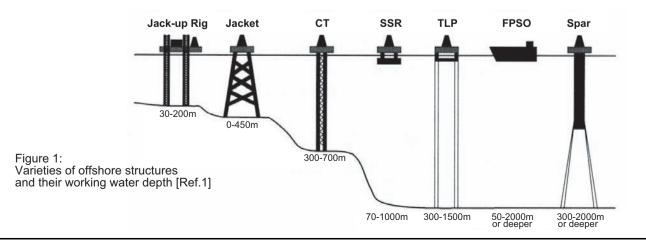
costs during construction. As shown in Figure 1 the maximum working water depth is 450 m for jackets due to the characteristic waving period.
