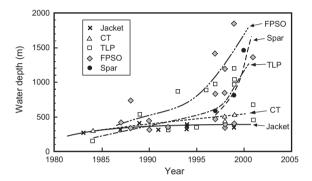
Figure 2: Water depth transition for offshore structures [Ref.1]
