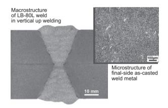
Figure 2: Typical macroscopic and microscopic structures of LB-80L weld (Refer to Figure 1 for welding conditions).
