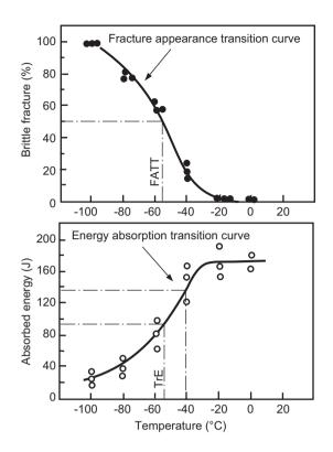
Figure 1: Energy absorption transition and fracture appearance transition curves of mild steel or low alloy steel welds.
