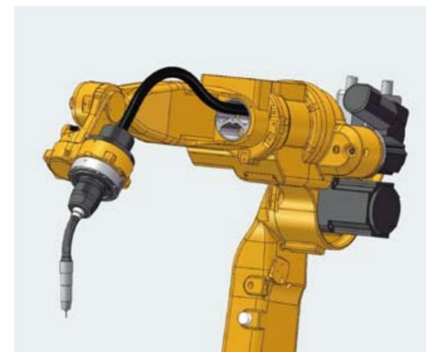
For the cable-integrated upper arm type, a wire feeder is mounted at the rear side of the upper arm; the torch cables extend from the wire feeder through the cable hole that runs alongside the upper arm. The torch body is supported at the wrist axis.
