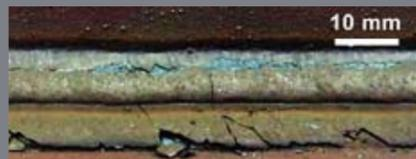
In multi-layer fillet welding, the good slag removability of conventional FCWs, means that the succeeding bead is apt to exhibit irregular toes because the slag of the preceding bead peels off naturally (Figure 2). Such a good characteristic, however, can adversely affect the formation of the succeeding bead without adequate support for it.
