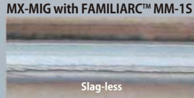
After electro deposition coating & corrosion test
