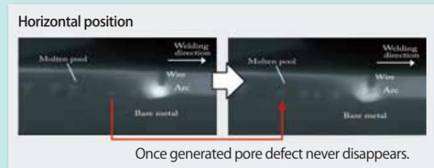
When Zn gas evaporates from just under the arc, bubbles do not form in the molten pool and pore defects are avoided. Accordingly it is now clear that the amount of pressure applied to the molten pool right under the arc is the dominant factor allowing Zn gas to evaporate quickly.
