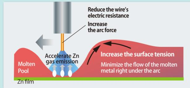
MIX-Zn solid wire was developed to optimize surface tension as well as to apply a higher current with the same deposition amount by reducing the wire's electric resistance.
