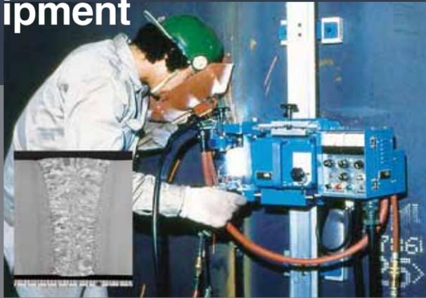
SEGARC™ (Simple Electro-Gas ARC), developed by Kobe Steel, Ltd. in 1974, is an extremely efficient electro-gas arc welding process in the vertical upward position. Even though about 40 years have passed since its debut, it continues to be applied in such fields as shipbuilding, crude oil tank fabrication and steel-frame building construction. It offers the following advantages:
