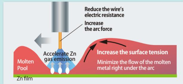
MIX-Zn solid wire was developed to optimize surface tension as well as to apply a higher current with the same deposition amount by reducing the wire's electric resistance.
