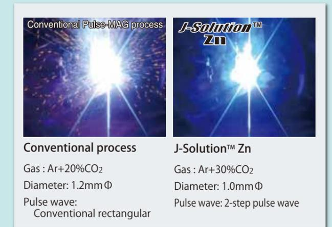
In summary, J-Solution™ Zn represents a new concept in welding procedures that both improves porosity resistance and reduces spatter. While both aims may appear incompatible in a conventional method (i.e. decreasing porosity may increase spatter), the combination of 1.0 mm MIX-Zn, chemically formulated for galvanized steel sheets; Digital-Pulse DP400R, with added new control software and parameter; and Ar+30%CO<sub>2</sub> shielding gas allows both issues to be solved together.
