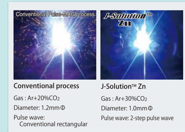
In summary, J-Solution™ Zn represents a new concept in welding procedures that both improves porosity resistance and reduces spatter. While both aims may appear incompatible in a conventional method (i.e. decreasing porosity may increase spatter), the combination of 1.0 mm MIX-Zn, chemically formulated for galvanized steel sheets; Digital-Pulse DP400R, with added new control software and parameter; and Ar+30%CO<sub>2</sub> shielding gas allows both issues to be solved together.
