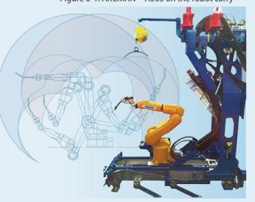
Figure 6-2: Actual welding operation with ARCMAN™ A30S at hull assembly
