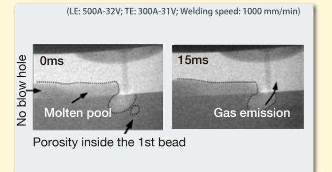
Figure 13: Mechanism of porosity reduction
