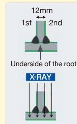
Figure 3: RT result in single- and tandem-electrodes welding processes
