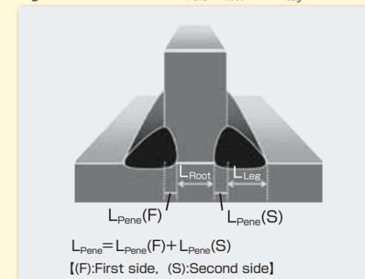
Figure 5 shows the relationship between the LE's torch angles and  $L_{Pene}$  (F), the penetration depth at the first side.
