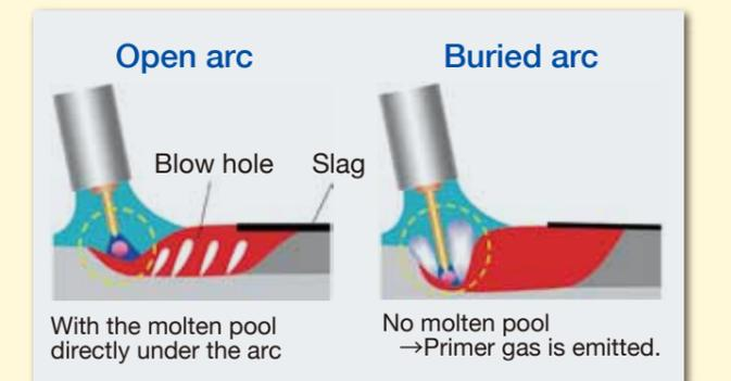
obtain a buried arc at the large welding current. Figure 15 shows the porosity resistance and shape of penetration, and Figure 16, the bead appearance by the HTM process. No porosity was generated at the first as well as second sides and excellent bead shape was also obtained.
