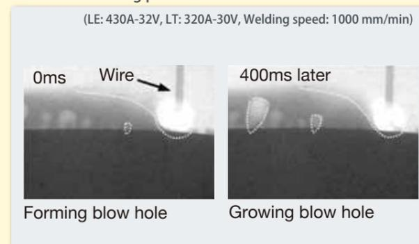
Figure 12: Observation of gas emission phenomenon by the newly developed process
