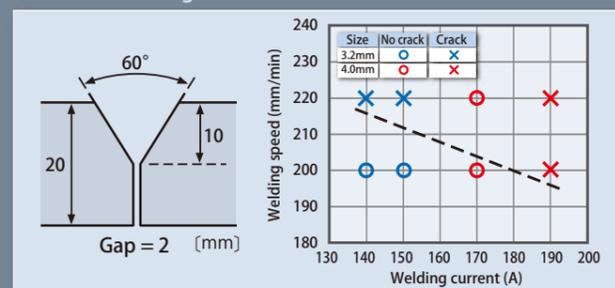
Because PREMIARC™ NI-C6J covered electrodes greatly reduce porosity generation, obtain superb hot crack resistance and fully satisfy the AWS requirements for 9% Ni steels, they are sure to fit your needs.
