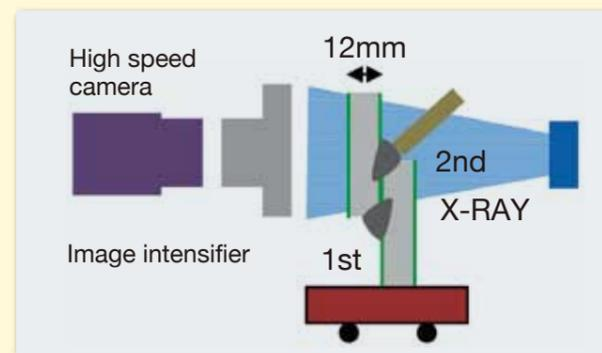
Figure 11: Formation of blow holes in a conventional welding process
