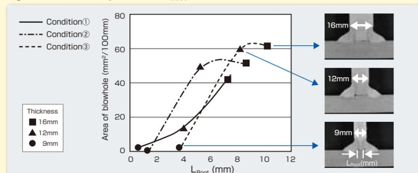
Figure 10: Observation method using X-ray transmission
