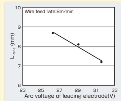
Figure 8: Relationship between  $L_{Pene}$  and the occurrence of blow holes
