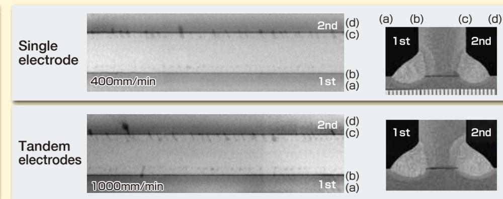
of blow holes can be observed in the fillet welds obtained from both welding processes; tellingly, the blow holes are initiated at the underside of the vertical member (hereinafter called the underside of the root) and appear in a line along the underside of the root. Also, more porosity appears at the second side than that at the first side because the evaporated gas emits only from the second side during welding as the first side is closed by the weld.
