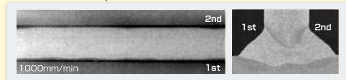
Figure 16: Bead appearance by the HTM process
