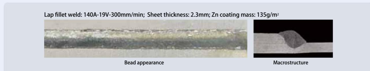
Figure 5: Bead appearance and cross-sectional macrostructure of **MX-100Z** (1.2mm dia.) weld
