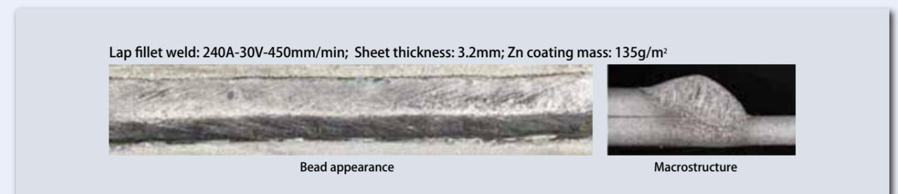
Figure 4: Bead appearance and cross-sectional macrostructure of MX-1Z (1.2mm dia.) weld
