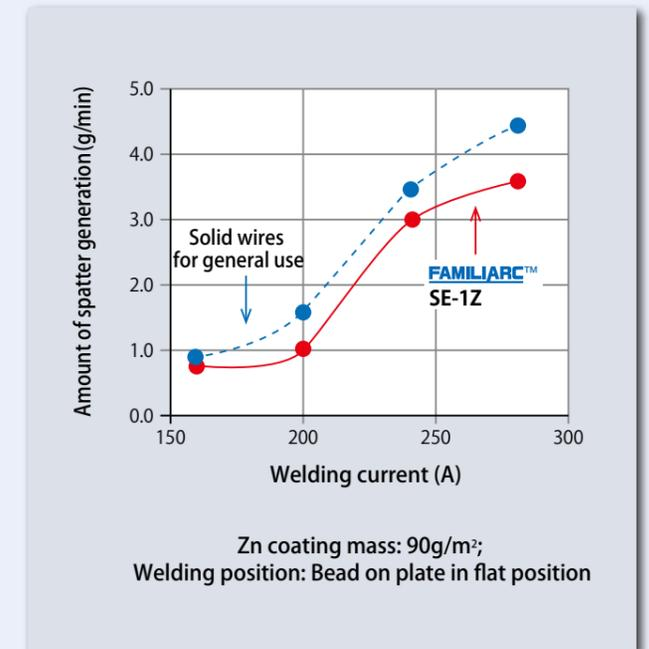
Figure 2: Comparison of spatter generation between SE-1Z and solid wires for general use
