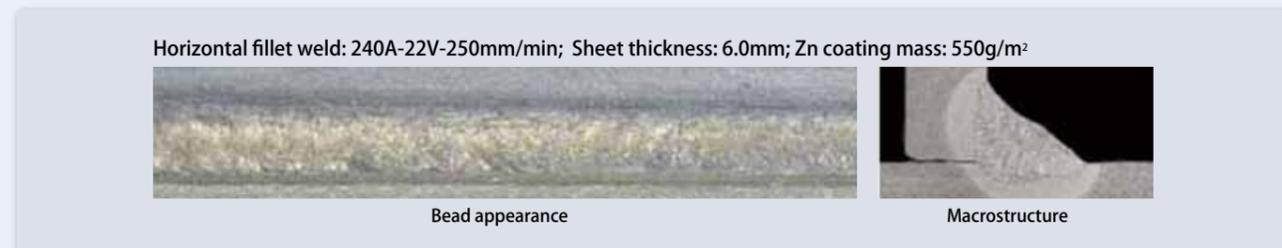
Figure 6: Bead appearance and cross-sectional macrostructure of **DW-1SZ** (1.4mm dia.) weld
