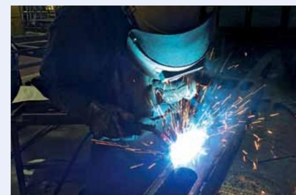
Figure 9: Welding a frame structure for a bus with **SE-1Z**
