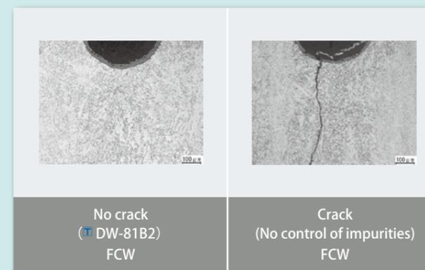
Figure 8: Observation of crack or no crack at U notch portion in C-shaped-ring cracking test
