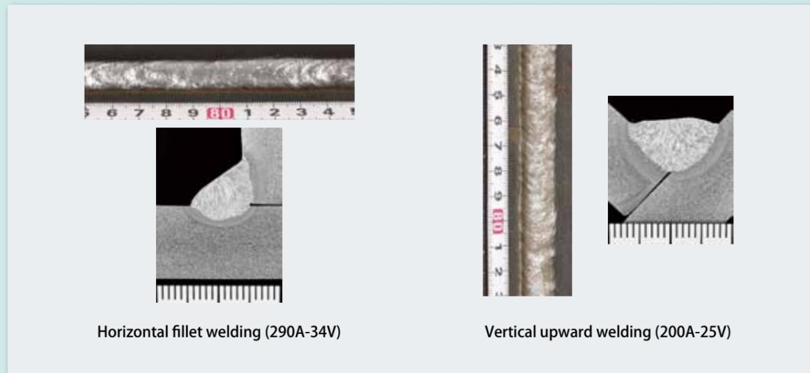
Figure 3: Bead appearances and cross-sectional macrostructures by welding positions
