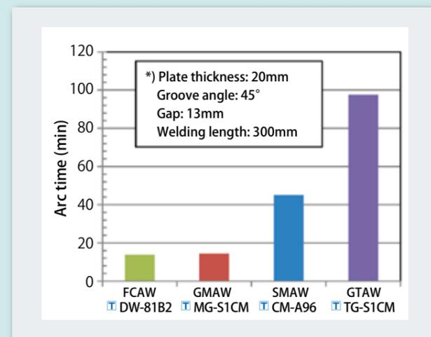
Figure 1: Comparison of arc time by welding processes
