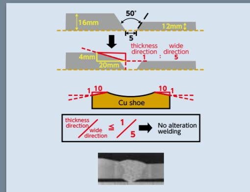
Figure 3: Application to a tapered joint & cross-sectional macrostructure of a tapered joint
