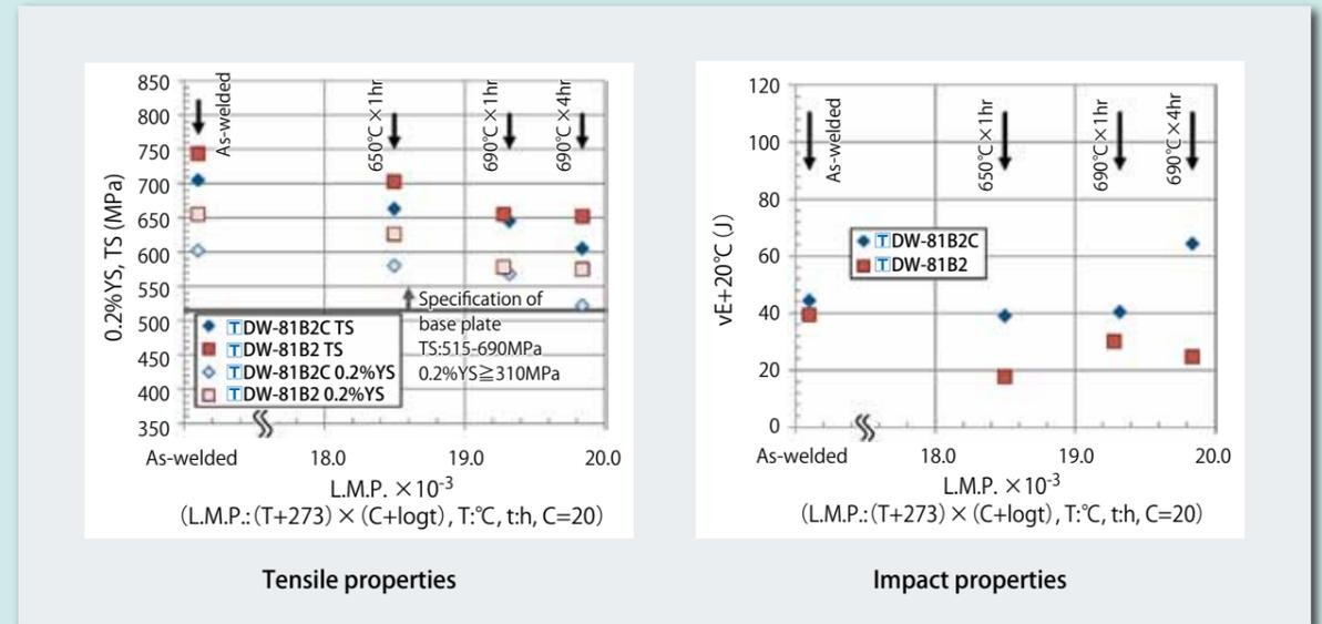
Figure 4: Tensile and impact properties of FCWs for 1.25Cr-0.5Mo heat resistant steels after PWHT
