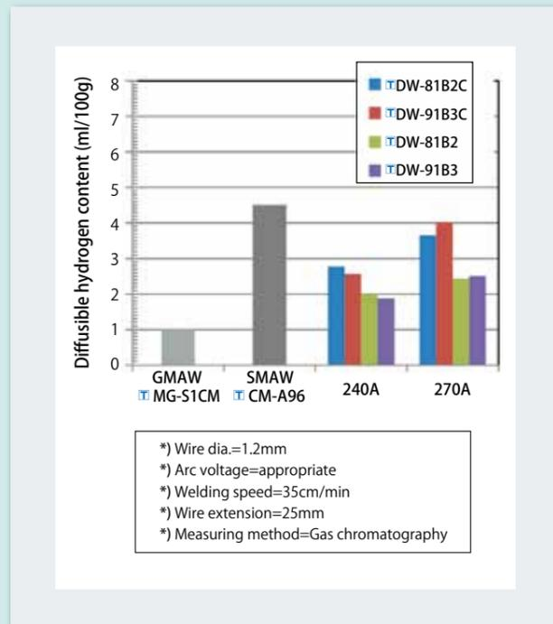
Figure 6: Diffusible hydrogen content of weld metal
