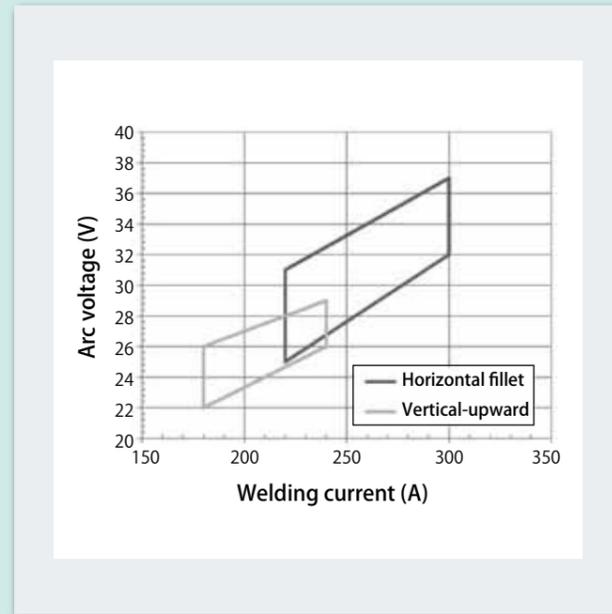
Figure 2: Applicable ranges of welding current and arc voltage by welding positions
