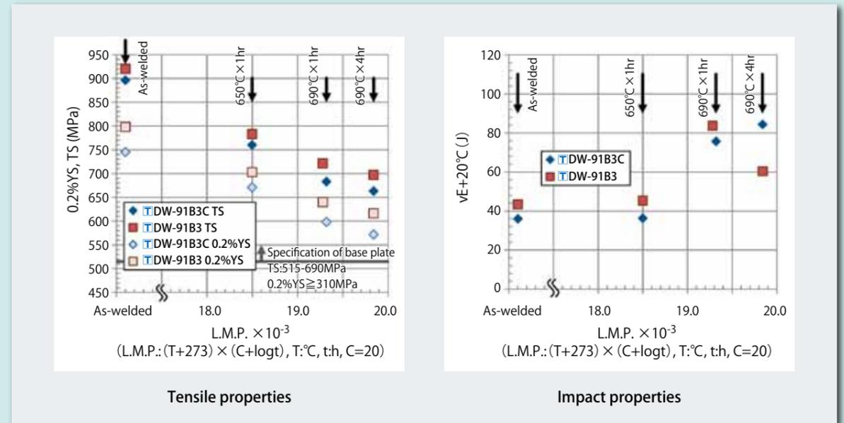
Figure 5: Tensile and impact properties of FCWs for 2.25Cr-1Mo heat resistant steels after PWHT
