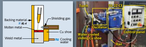
Figure 1: Schematic diagram of SEGARC™ process
