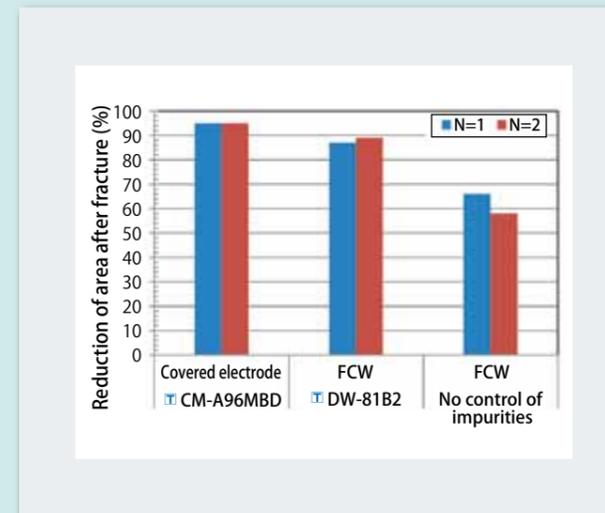
Figure 7: Comparison of reduction of area after fracture in high temperature-slow strain rate-tensile test
