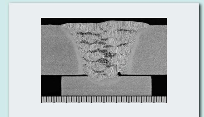
Figure 9: Cross-sectional macrostructure showing ferrite band generation (PWHT:  $710^\circ C \times 24h$ )
