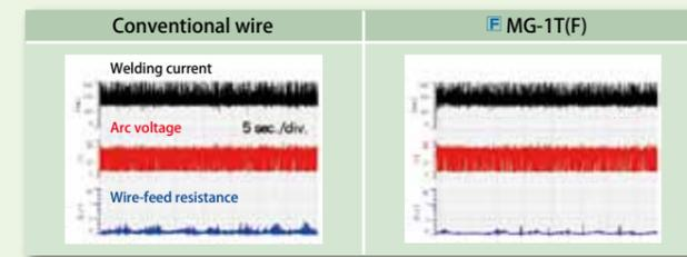
Figure 6: Time variation of welding current, arc voltage and wire feed resistance between a conventional wire and MG-1T(F)
