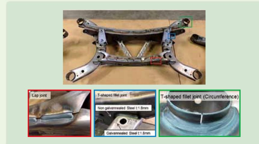
Figure 13: Appearance and welds of suspension cross-members
