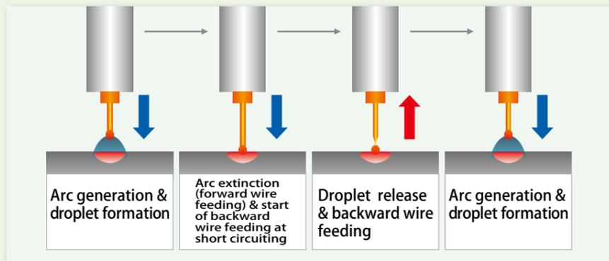
Figure 3: Wire feeding control method
