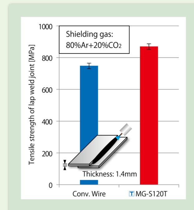
Figure 1: Comparison of tensile strength of lap joints welded with conventional (JIS Z 3312 YGW16) and TRUSTARC MG-S120T wires on 980MPa class steel sheets
