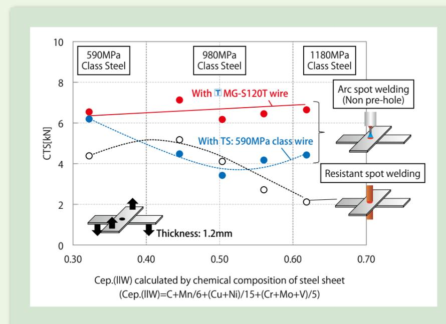
Figure 2: Influence of tensile strength of steel sheet, carbon equivalent, welding method and consumable wire on cross tensile strength
