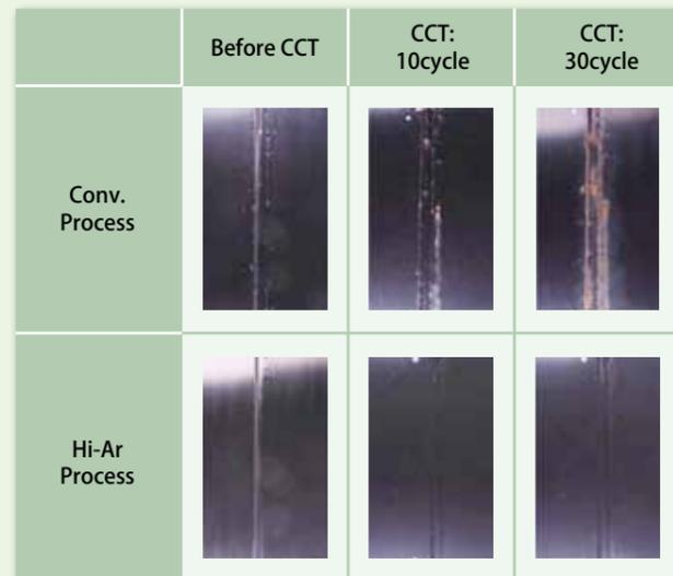
Figure 10: Comparison of corrosion resistance between conventional and Hi-Ar processes
