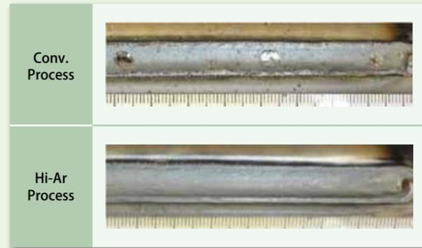
Figure 9: Comparison of bead appearance between 80%Ar-20%CO<sub>2</sub> shielding gas (conventional process) and Hi-Ar Process
