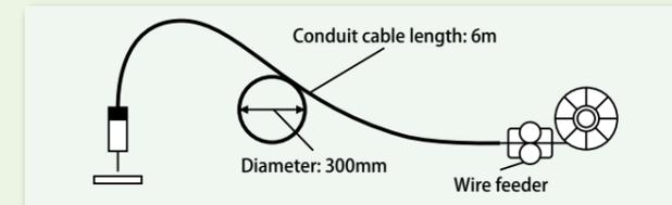
Figure 5: Schematic drawing of wire feeding test
