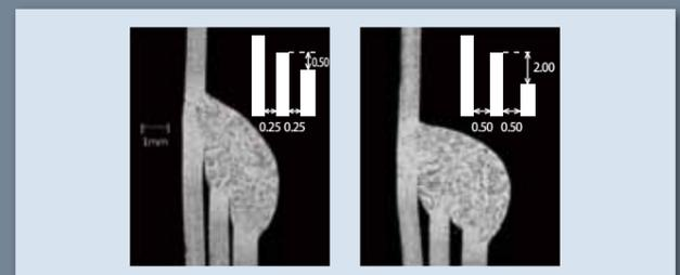
Figure 3: Examples of gap resistance evaluation with PREMIARC MX-T430Nb
