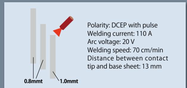
Figure 2: Welding condition
