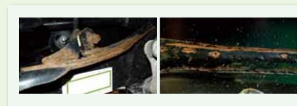
Figure 7: Rust generated on suspension components and weld bead appearance
