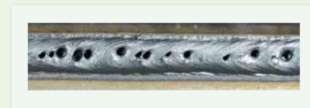
Figure 8: Porosity defects generated on a weld bead
