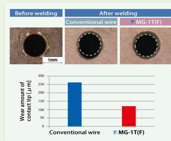
Figure 4: Comparison of wear at the contact tip
