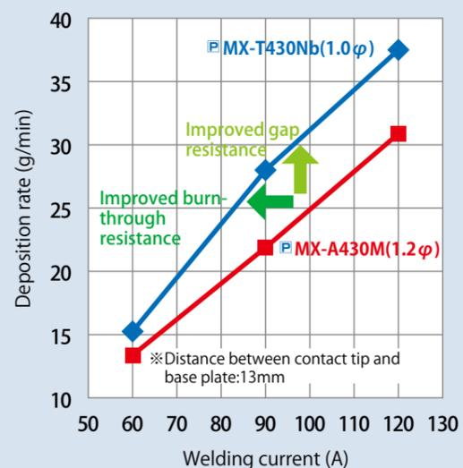
Figure 1: Relationship between welding current and deposition rate
