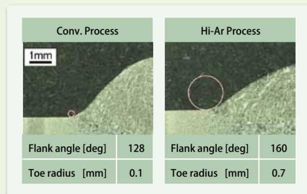
Figure 11: Comparison of toe shapes
