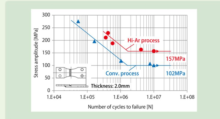
Figure 12: Results of fatigue test ※Stress ratio=0, Frequency=25Hz
