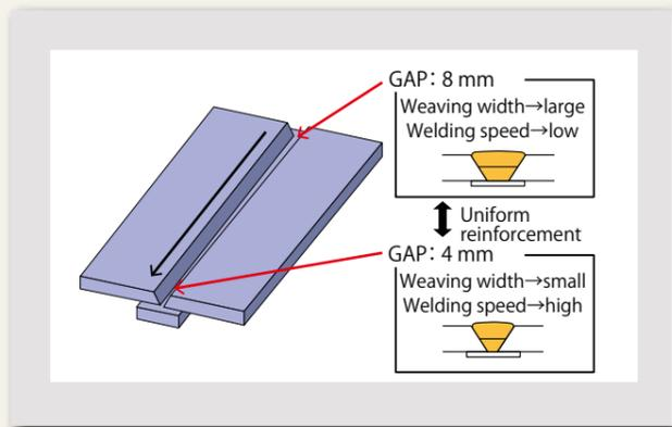
Figure 10: Root gap sensing function
