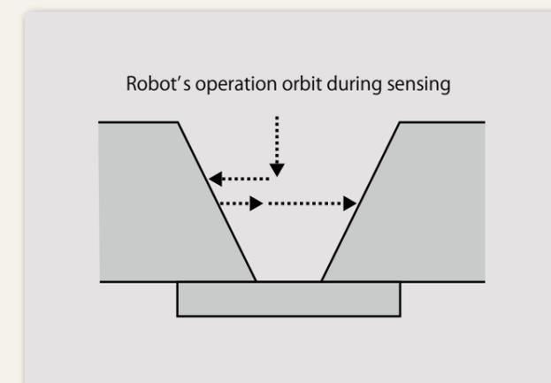
Figure 4: Root gap measurement by touch sensing method
