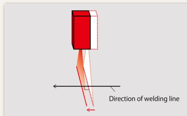
Figure 6: Laser sensor scanning operation
