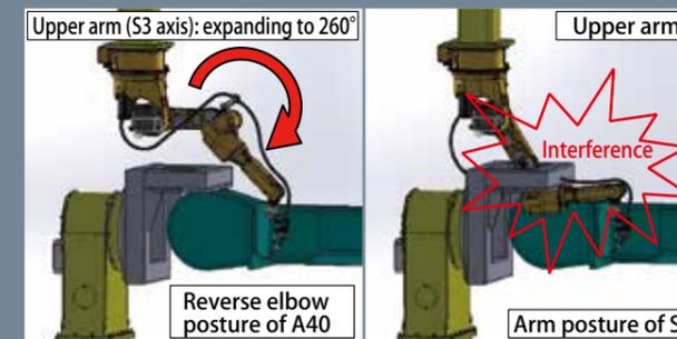
Figure 6: Ways that an overhead welding robot can approach a workpiece
