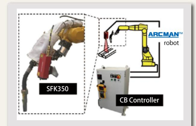
Figure 7: Laser Sensing System components
