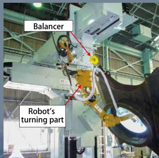
Figure 4: Placement of torch cable on the SR robot
