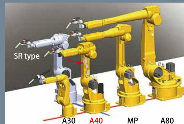
Figure 2: ARC MAN™ Series line-up
