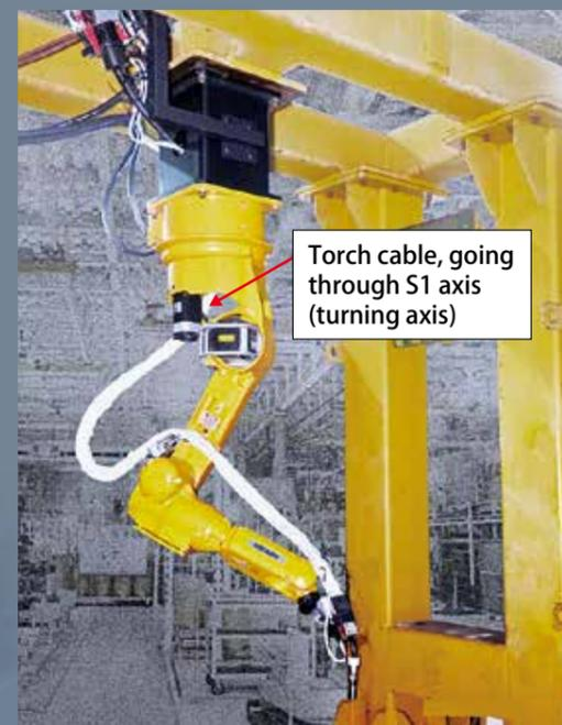
Figure 5: How a torch cable is treated on the A40 robot
