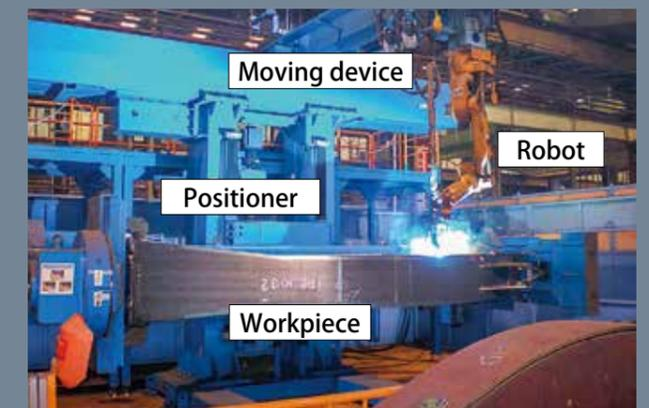
Figure 3: A typical welding system
