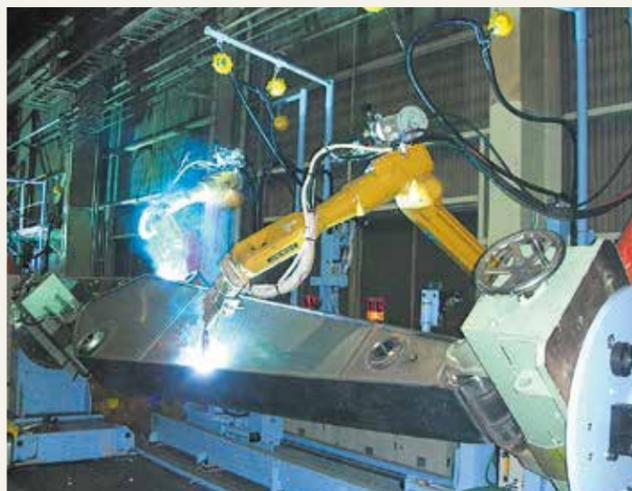
Figure 2: ARCMAN™ robot welding system for arm of construction machinery
