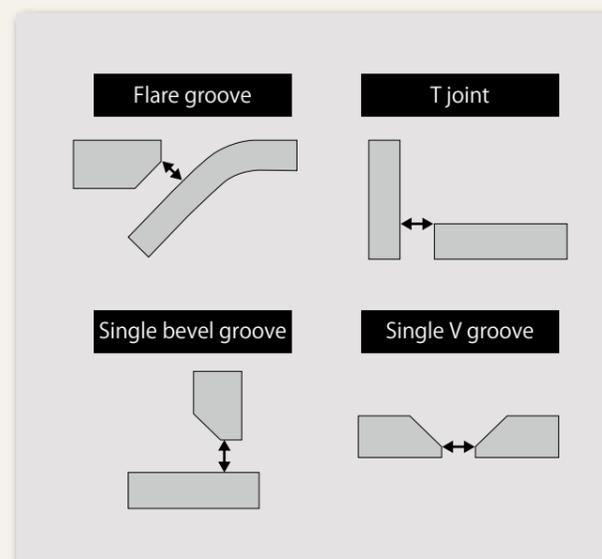
Figure 3: Groove shapes applicable to detection by laser sensing
