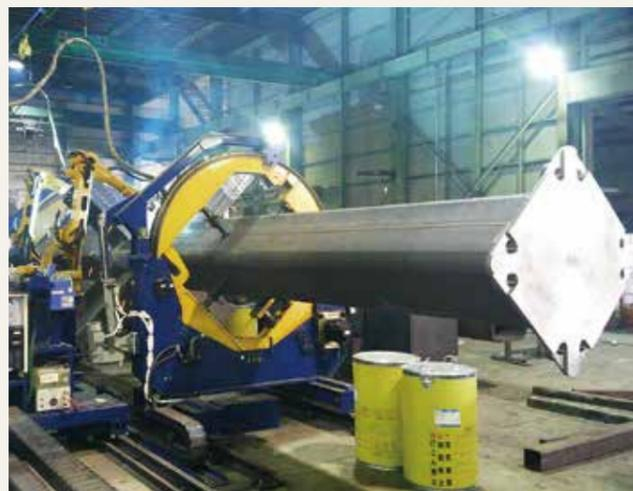
Figure 1: ARCMAN™ structural steel large assembly "2-arc" robotic welding system
