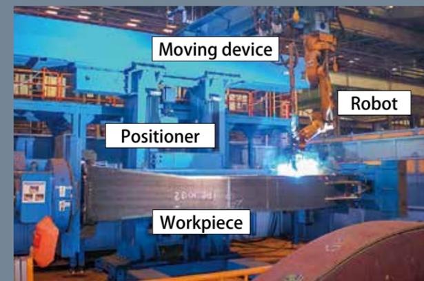
Figure 3: A typical welding system
