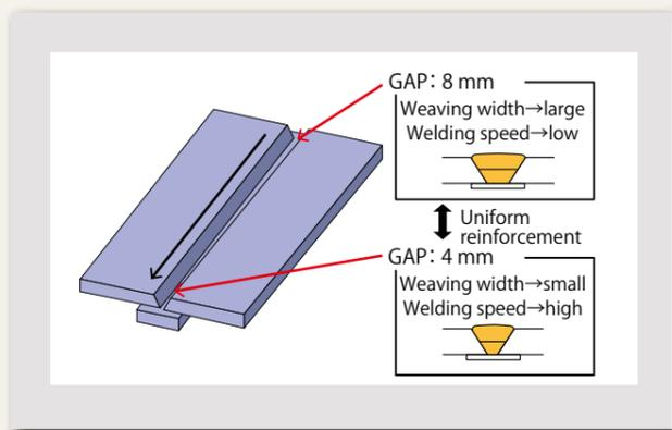
Figure 10: Root gap sensing function
