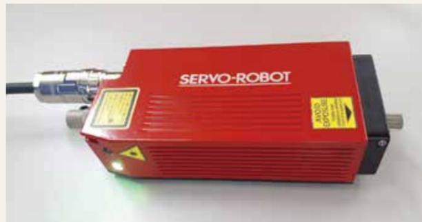
Figure 5: The custom-made SFK350 Laser Sensor
