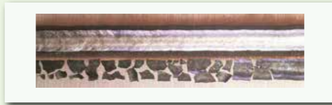
Figure 1: Easy slag removal and beautiful bead appearance right after welding of DW-308L
