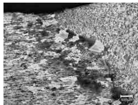
Figure 4: Grain growth in HAZ of ferritic stainless steel
