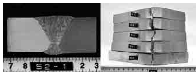
Figure 11: Macrostructure and side bend test results of a dissimilar joint welded by type 309
