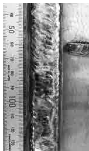
Figure 4: Bead appearance of DW-410NiMo
