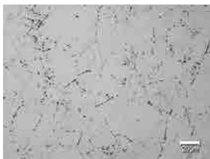
Figure 1: Cr carbide precipitations in stainless steel
