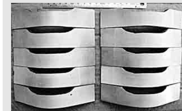
Figure 3: Hot crack test result by side bend test *1 ND: No Defect
