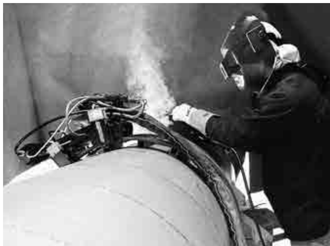
Figure 6: Welding of clad pipe by DW-N625P and Magnatech machine.
