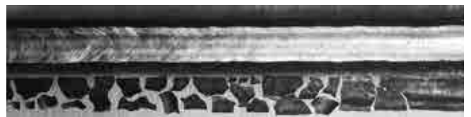
Figure 11: Bead appearance of DW-308L horizontal fillet welding by DW-308L
