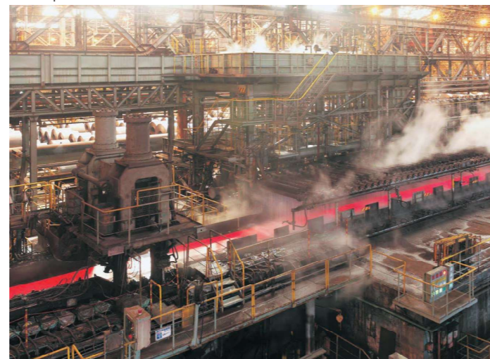
Laminar Cooling Facilities
