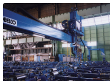
片面板継サブマージ / 溶接装置 One-Side SAW Welding Process
