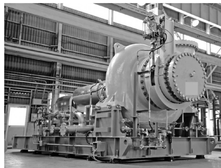
図6 PDH用ターボ圧縮機 Fig.6 Centrifugal compressor for PDH application
