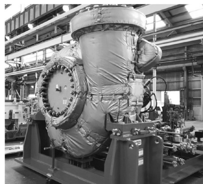
図5 EO/EG用ターボ圧縮機 Fig.5 Centrifugal compressor for EO/EG application
