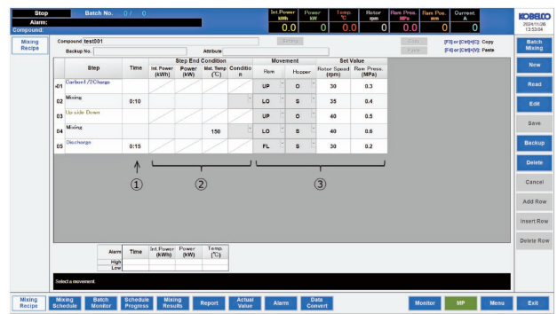
図2 混練条件設定画面 Fig.2 Mixing condition setting screen
