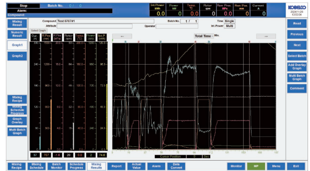
図3 混練結果画面 Fig.3 Mixing result screen
