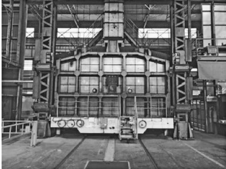
図12 改造予定の加熱炉 Fig.12 Heating furnace scheduled for modification
