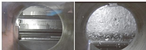
Propane condensation on E2 heat transfer tube
