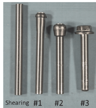
図8 ボルト外観 Fig.8 Appearance of trial-produced bolts
