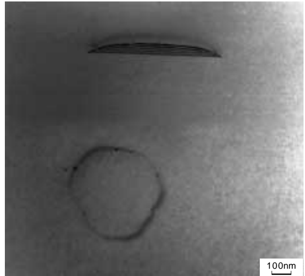
写真 1 化合物半導体単結晶中の積層欠陥 Photo 1 TEM image of defect in compound semiconductor crystal
