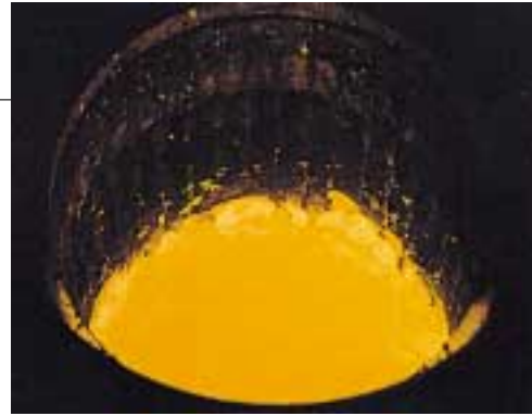
a) Appearance of Melting Ti
