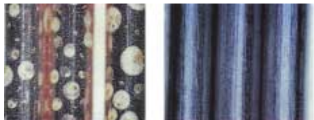
(a) Conventional Cu-coated solid wire (b) Non-Cu-coated solid wire
