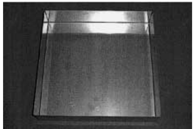
c) Stainless steel press-formed after KENI FINE coating
