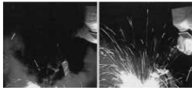
a) Metal Type FCW b) Solid Wire Comparison of spatter emission state
