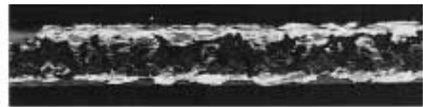
Slag appearance on the bead
