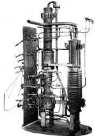
写真 2 絶縁管内構造 Photo 2 Structure, insulation materials removed
