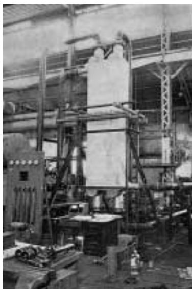
写真7 性能テスト中の ALEX Photo 7 Heat exchanger "ALEX" under performance test
