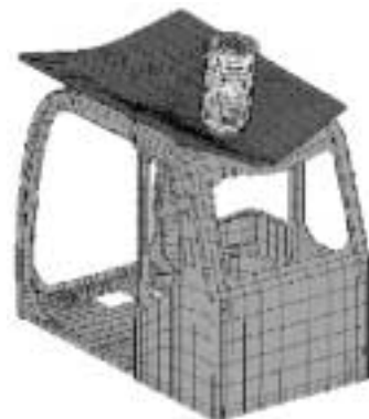
図7 油圧ショベルキャブの落下衝撃解析 Fig. 7 Impact analysis of backhoe cabin subject to falling object
