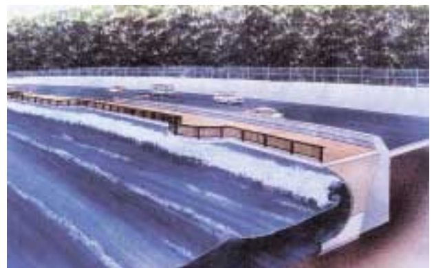
図12 フレア護岸 Fig.12 Flaring shaped seawall
