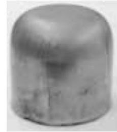
図12 開発鋼の深絞り成形性 Fig.12 Deep drawability of the developed steel
