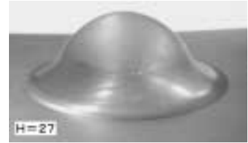
図11 開発鋼の張出し成形性 Fig.11 Bulging formability of the developed steel
