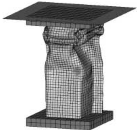
図5 角筒の変形形状 Fig. 5 Result of FEM simulation
