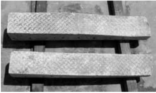
写真1 縞鋼板の突起痕 Photo 1 Trace of steel checker plate
