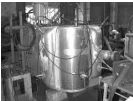
写真 2 疲労試験用大型コアの外観 Photo 2 Outside view of testing apparatus of large size core for fatigue test
