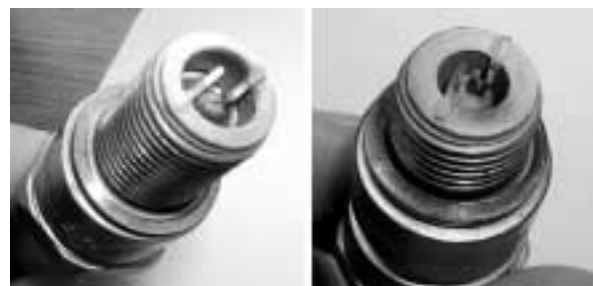
写真5 点火プラグ（左：精製装置設置前、右：精製装置設置後） Photo 5 Spark plug (Left : Before installation of gas pretreatment unit, Right : After installation of gas pretreatment unit)
