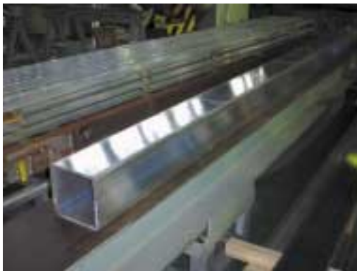
(b) 1mass%B-A3004 extruded pipe
