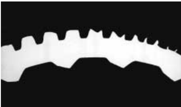
写真 3 ECHT19fpi の管軸直角断面 Photo 3 Cross-sectional view of ECHT19fpi (Cut in round slice)
